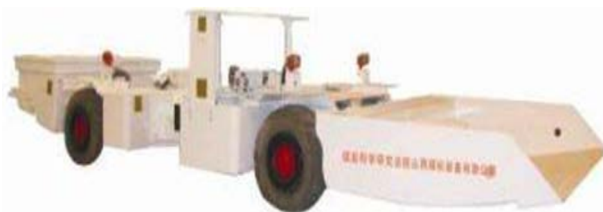
Figure 4. Domestic CLX3 type explosion-proof battery forklift.
