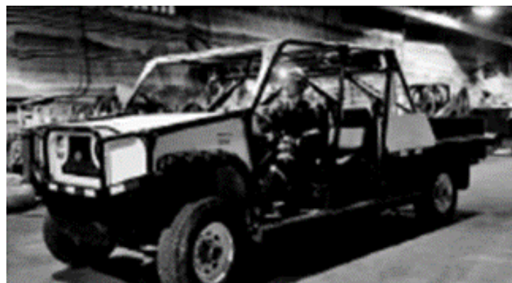
Figure 3. The truss-type underground explosion-proof light passenger vehicle.
